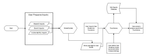
Figure 1. High-level workflow for using Model Builder
